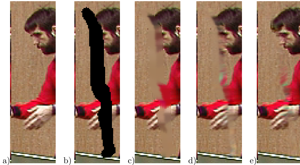
Figure 6.3: Scratch "tmask1" (b) restoration in frame No.78 from the "tennis" sequence (a)original frame-cut (b)corruption by the scratch (c)Median Filter (d)3D CAR model (e)3.5D CAR model.
