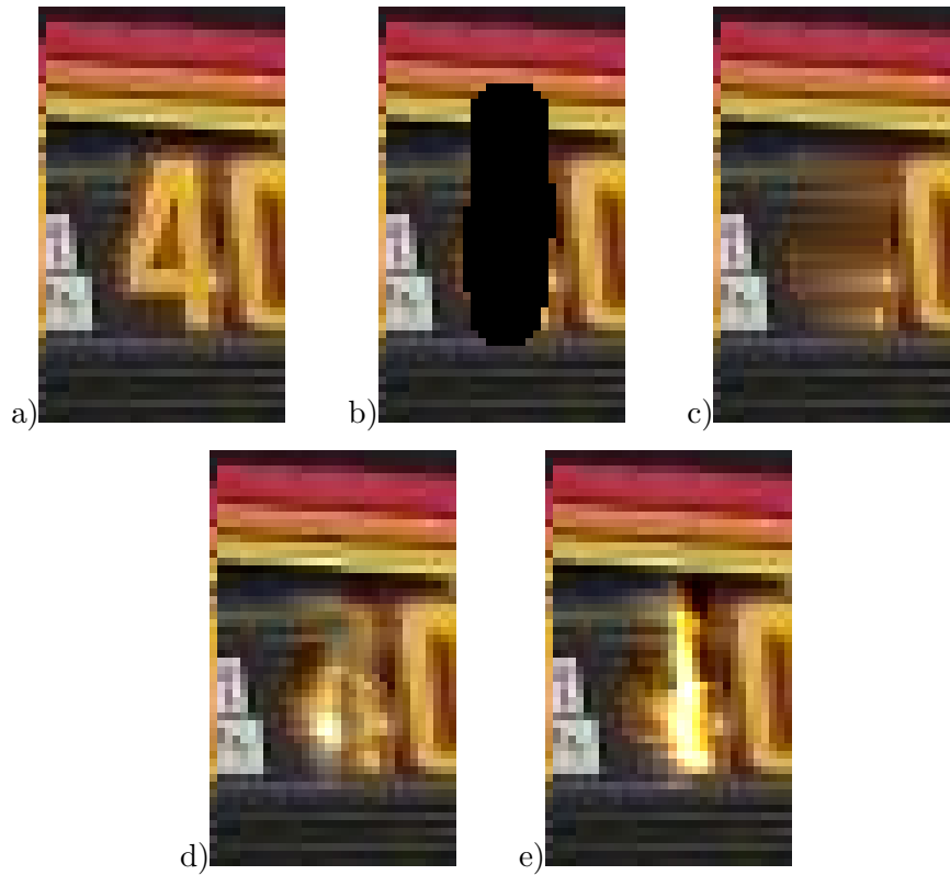
Figure 6.8: Scratch “mask4” (b) restoration in frame No.77 from “cars” sequence (a)original frame-cut (b)corruption by the scratch (c)Linear Regression (d)3D CAR model (e)3.5D CAR model without MC.
