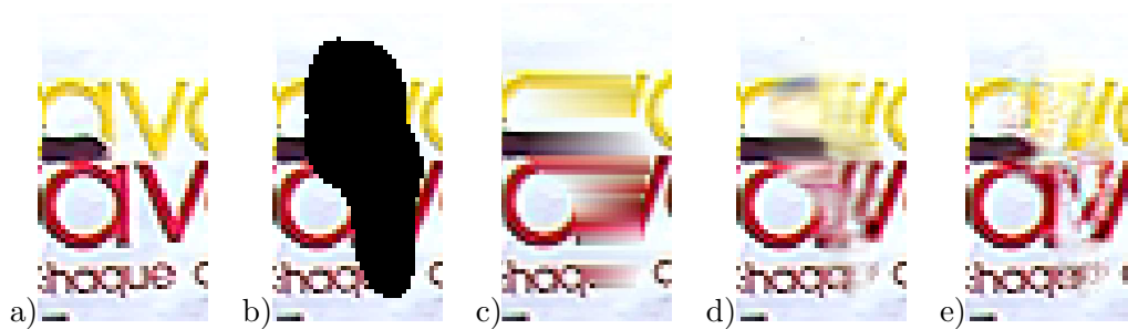
Figure 6.5: Scratch “tmask3” (b) restoration in frame No.78 from the “tennis” sequence (a)original frame-cut (b)corruption by the scratch (c)Linear Regression (d)3D CAR model (e)3.5D CAR model.
