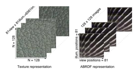
**Figure 2.4:** Two common BTF representations - *Texture representation* (left) and *ABRDF representation* (right).
