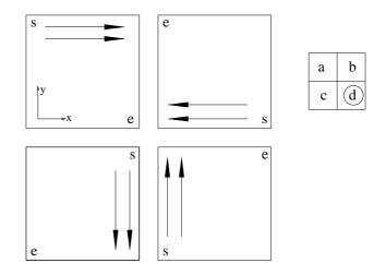
**Figure 5.4:** Directions of scanning in four different scans through array of normals and used contextual neighbourhood.
