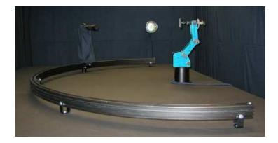
Figure 3.4: BTF measurement setup of Bonn University.
