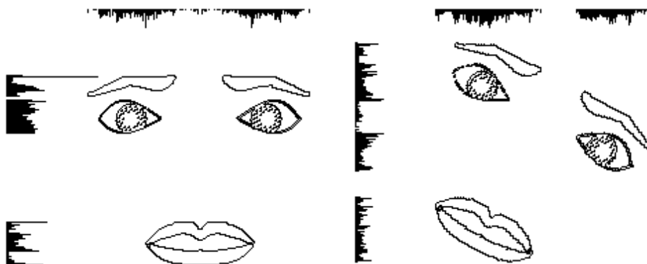
Figure 4.3: Two examples of using edge detection for recognising the angle of rotation of an image
