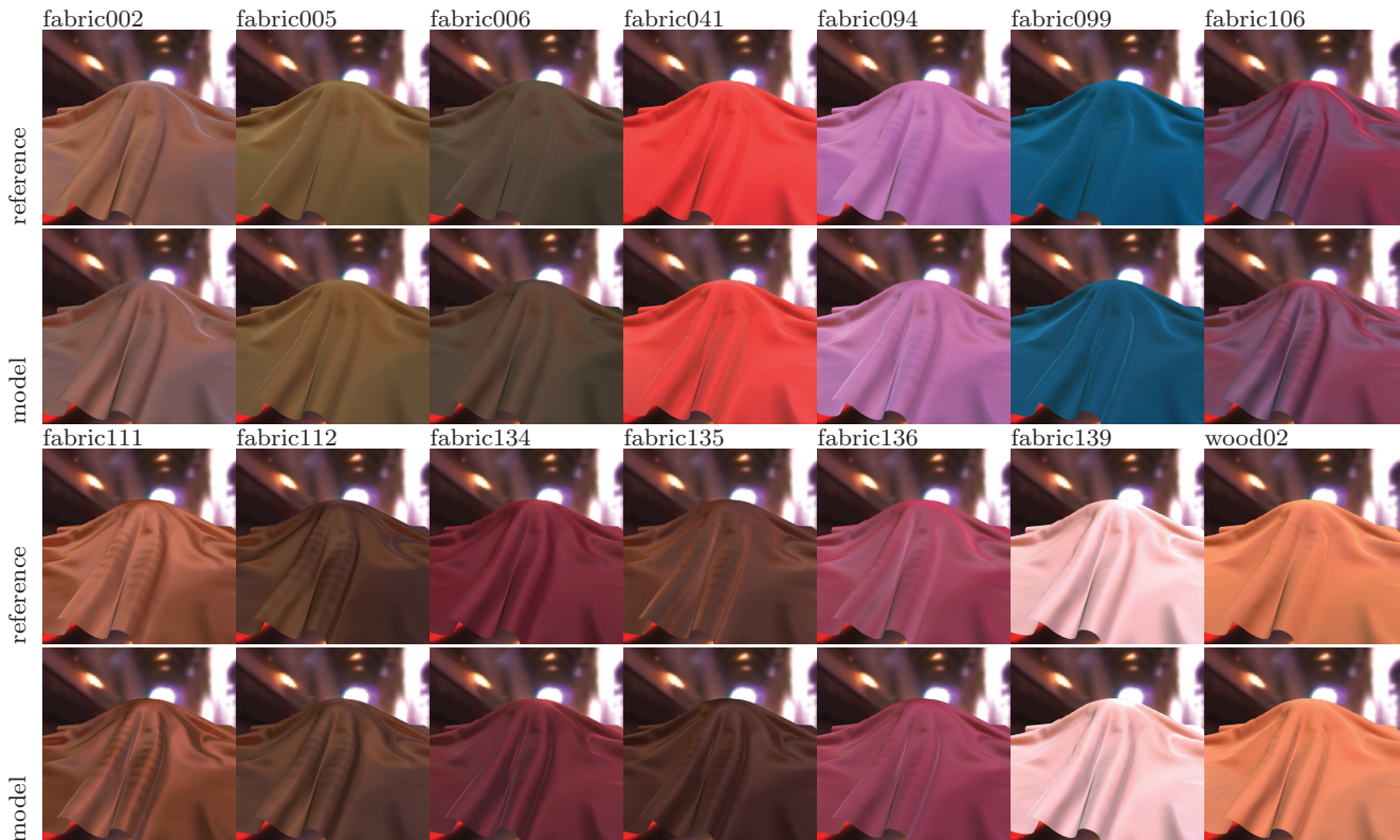
Fig. 15 Comparison between reference BRDF (odd rows) and proposed BRDF model (even rows) renderings in grace illumination environment for 14 tested BRDFs.
