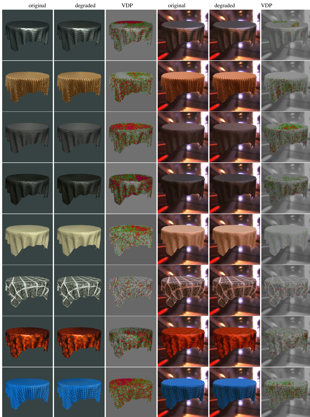
Figure 5: Renderings of degraded images visually equivalent with original BTF, for pointlight (first column) and grace (second column) environment for all tested samples. Corresponding visual difference predictor result is shown in third column, respectively.
